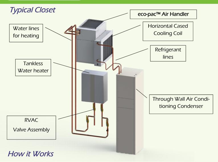
The eco-pac™ air handler uses heat from the water heater or boiler for space heating and accommodates conventional air conditioning for summer cooling. The compact size of the smaller unit allows for closet installation of all components where space is at a premium. The larger units are used in bigger homes where more capacity is needed. The high efficiency EC motor in the eco-pac™ allows for multi-speed operation, giving you both ultimate comfort and great energy savings.
