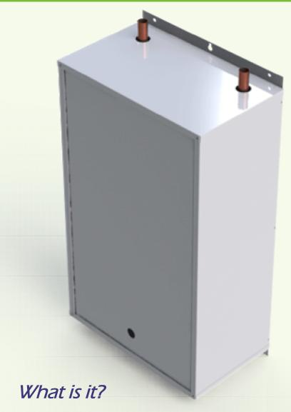
The TMM™ is a self contained package used for radiant floor heating of up to 5 zones. It contains a pump for each zone, a temperature control mixing valve, and electronic controls inside of an attractive white cabinet for a clean and compact installation.
