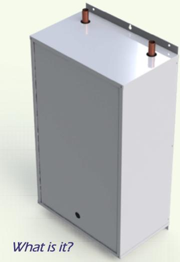
The TMMD™ is a self contained package designed to be connected directly to a tankless water heater and used for radiant floor heating of up to 5 zones. It contains a primary pump, a pump for each zone, a temperature control mixing valve, and electronic controls inside of an attractive white cabinet for a clean and compact install.
