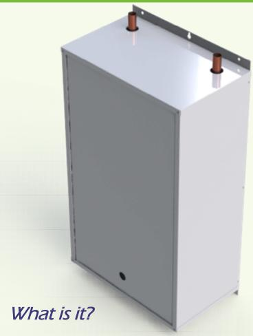
The TMMX™ is a self contained package with a heat exchanger used for radiant floor heating for up to 4 zones. The heat exchanger is used to separate the in-floor heating from the hot water source. Suitable for glycol systems or domestic hot water. It contains a primary pump, a pump for each zone, a temperature control mixing valve, a plate heat exchanger, and electronic controls inside of an attractive white cabinet.
