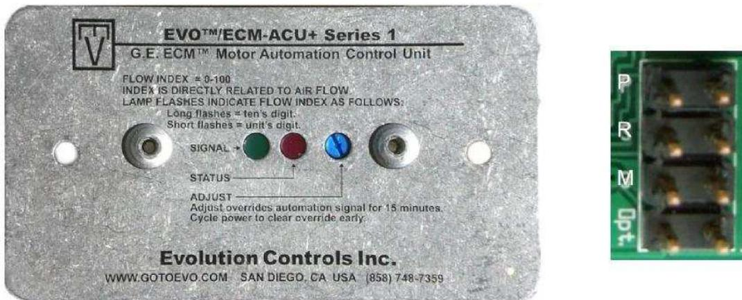
Note: The green signal light of the EVO motor control flashes according to its speed output to the motor. Ex. 5 long 3 short blinks = 53%
